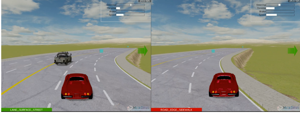
Fig. 6: Frames from two representative replays of MetaDrive’s “Scenario 605”, illustrating flaky behavior caused by nondeterministic scenario execution. The ego vehicle (a red sedan) takes two different paths in the final segment: in some repetitions it stays in the middle lane ( left image ), while in others it shifts to the right lane near the sidewalk ( right image ). When the vehicle moves close to the road edge, it collides with the sidewalk; when it remains in the middle lane, the scenario completes without any ego collision.
