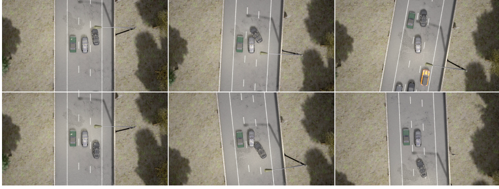
Fig. 5: Frames from two representative replays of CARLA Bench2Drive’s “Scenario 17563”, illustrating flaky behavior caused by nondeterministic scenario execution. The ego vehicle (a black sedan in the middle lane) encounters a cut-in scenario on a three-lane motorway. Columns correspond to time progression: the left, center, and right columns show the system state at times t_0 , t_1 , and t_2 , respectively, where consecutive frames are separated by one second. Rows correspond to different replays. Due to nondeterministic behavior of the background vehicle to the right of the ego, the cut-in scenario unfolds differently across replays. In the first replay ( top row ), the adversary vehicle accelerates ahead of the ego and cuts into its lane, resulting in a severe collision that forces the ego vehicle to stop and fail the scenario. In the second replay ( bottom row ), the adversary vehicle remains behind the ego at the time of the cut-in, leading to a collision with lower relative velocity that allows the ego vehicle to recover and complete the scenario with no further violations.
