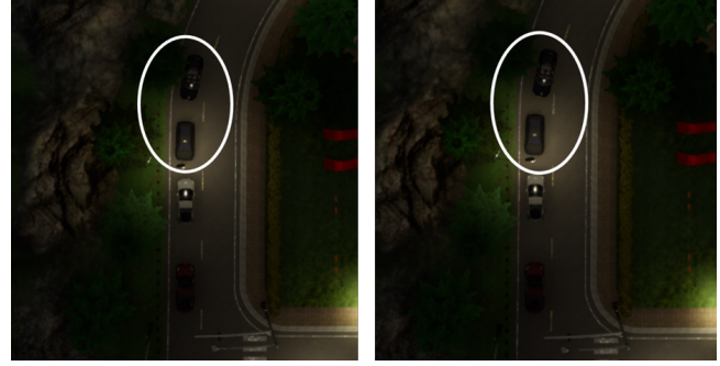
Figure 3: Counterfactual replay results. TransFuser++ (left) maintains its baseline behaviour despite reduced visibility, whereas TransFuser (right) avoids the collision observed in the original scenario, demonstrating a distinct response to environmental modifications.
